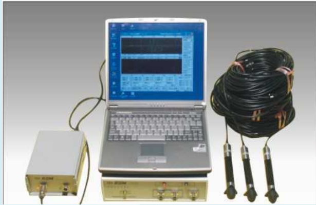
Acoustic wave (single or cross-hole method)
