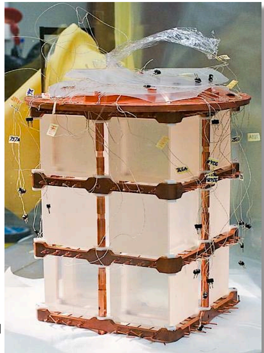
A miniature CUORE -like tower containing 12 \text{TeO}_2 crystal detectors. All of the copper parts were coated with a 50-micron-thick Parylene film prior to assembly.
