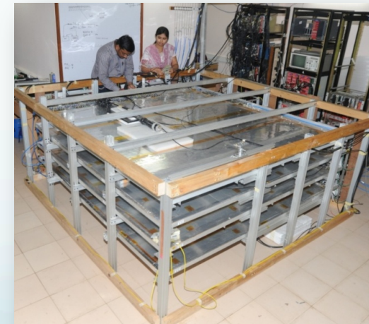
2m x 2m glass RPC test stand
