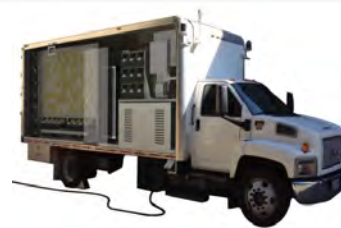
Figure 1 A cutaway view of the RadMAP vehicle showing the radiation sensors inside.
