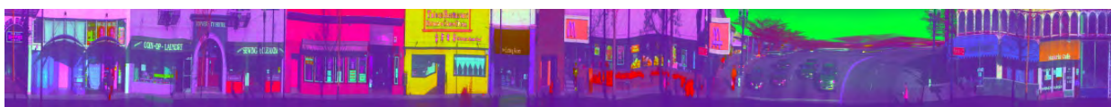
A false color hyperspectral image taken in downtown Berkeley. Each pixel has hundreds of times the color information of a typical RGB image and can be used to identify materials near the vehicle.
