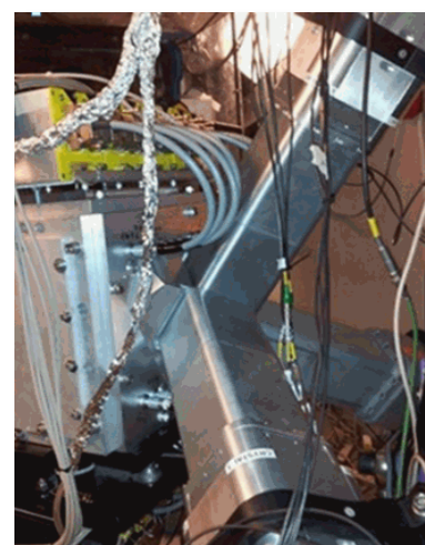
The new Berkeley Gas-filled Separator focal plane detector called C3 (Clover-Corner-Cube) was built in the shape of the corner of a cube. Each of the 3 faces of the cube are occupied by a 64 \times 64 \text{ mm}^2 DSSD and a similar-sized punch-through detector.
