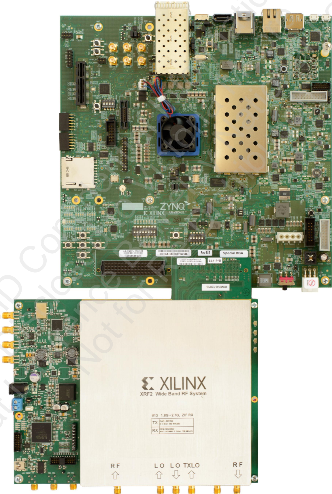
Figure 8: ZCU102 with AMD RF Kit v2.0
