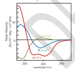
Poly-L-lysine in three conformations: alpha helix, b-sheet and random coil. Far-UV region of the CD spectra reveal peaks characteristic of these secondary structure elements, with helices having negative peaks at 222 nm and 208 nm and a positive peak around 190 nm,  $\beta$ -sheet proteins have a negative peak around 218 and a positive peak around 195 nm, and a random coil has a negative peak around 200 nm (as does poly-proline II helix).
