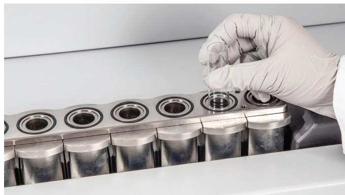
Figure 13. Inserting a glass liner—step 1.
