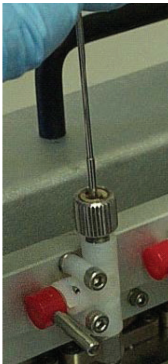
Figure 88. Inserting the needle into the guide adapter.
