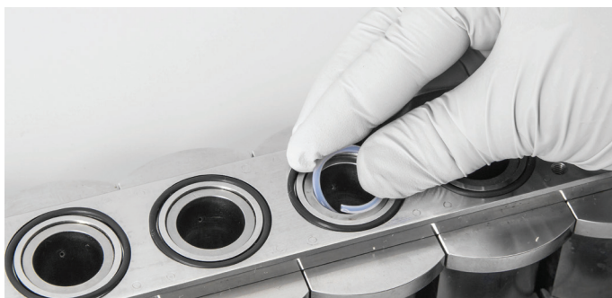
Figure 64. Insertion of the glass liner gripper.
