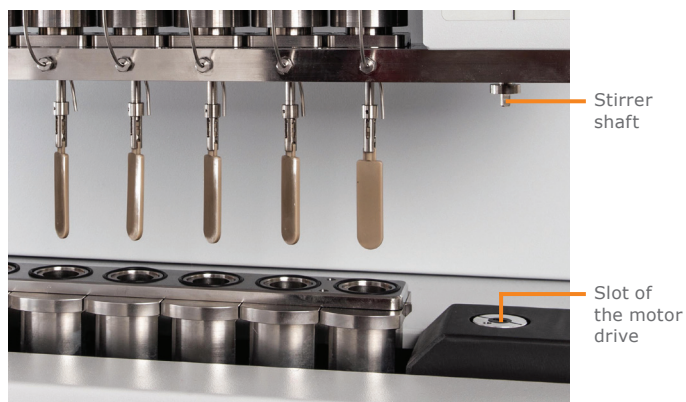
Figure 16. Placing the stirrer assembly.
