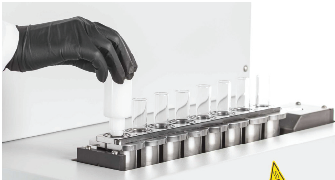
Figure 15. Inserting a glass liner—step 3.
