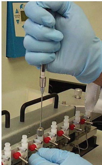
Figure 90. Closing the valve.
