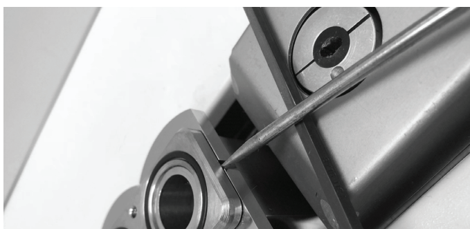
Figure 59. Leveraging the screwdriver.
