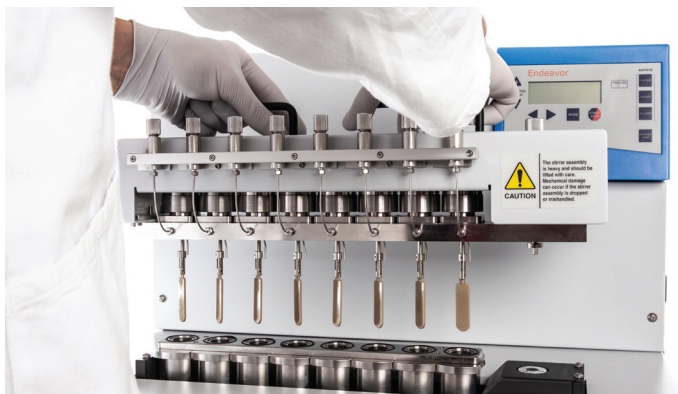
Figure 8. Removing the stirrer assembly.
