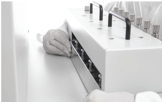
Figure 20. Fitting the rear clamp.
