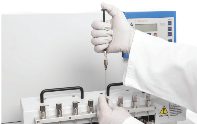
Figure 37. Injecting into a pressurized RV.
