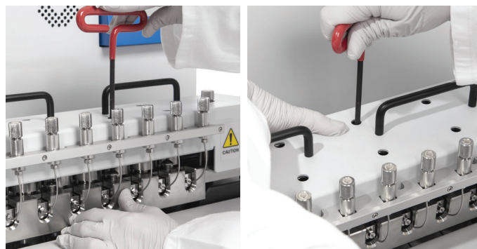
Figure 22. Tightening the front clamp (left) and rear clamp (right).
