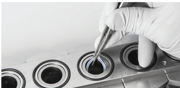
Figure 63. Removal of the glass liner gripper.
