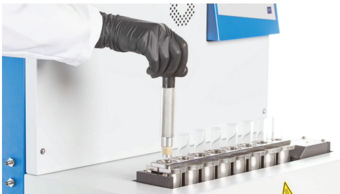
Figure 12. Inserting the glass liner removal tool.
