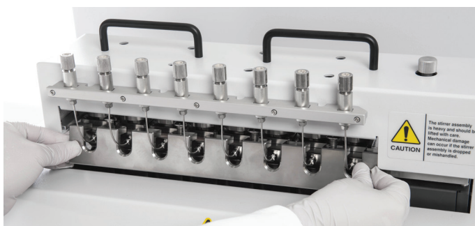
Figure 19. Fitting the front clamp.
