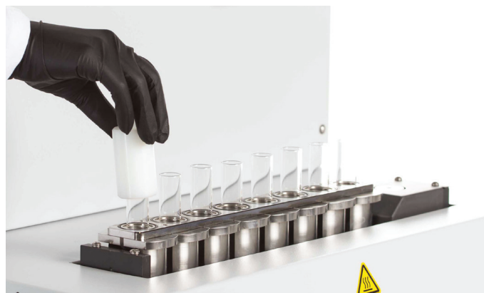
Figure 14. Inserting a glass liner—step 2.
