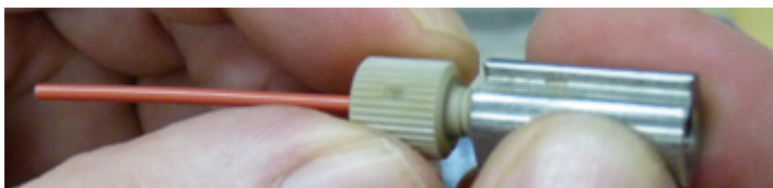
Figure 24 Red PEEK tubing into one end of slotted metal insert
