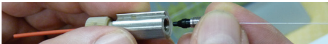
Figure 25 Screwing in the probe needle
