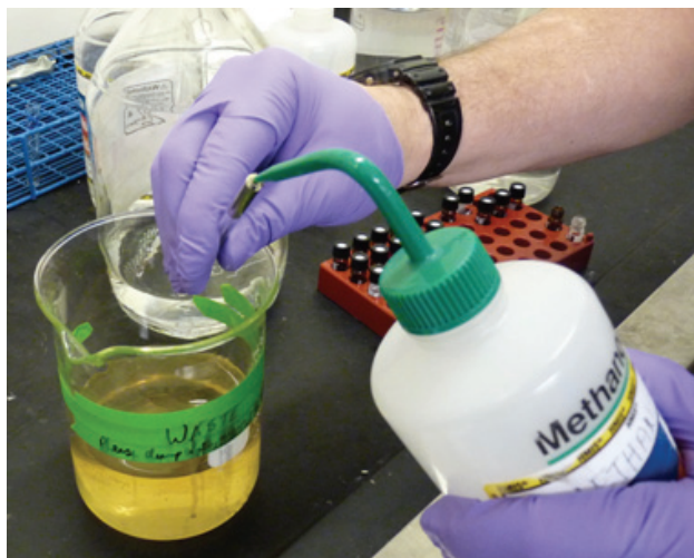
Figure 16 Cleaning the capillary under the hood
