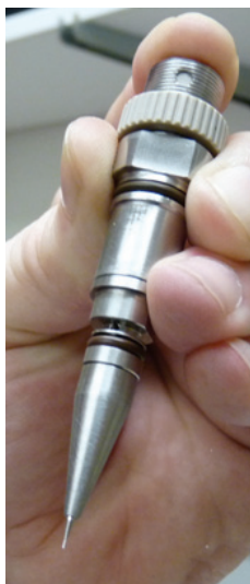
Figure 28 Needle is out 1/8 inch
