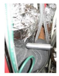
Many nuts and bolts are hard to access on the vacuum chamber. Sometimes they have to be assembled almost blind and the employee is forced to work with a bad posture. Special, ergonomically shaped tools (wrenches, pliers etc.) of different lengths are needed to help tightening these flanges in an easier way.
