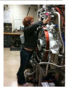
Portable cranes or crane carts are of high interest as well to help with the load of the parts which need to be attached (the turbo pump weighs about 30lbs; with stretched out arms it can hurt your back quickly).
