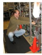
The flanges are hard to reach since the chamber is tall or located in the middle of a laser table. The employee has to tip-toe on the step stool, work with stretched out arms, or overhead. (Foldable) platforms and pedestals are needed to get the worker closer to the object. Longer tools (wrenches, pliers etc.) would help as well.
