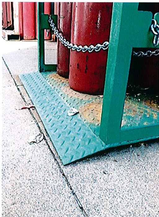
Angled transition can cause tank to fall
