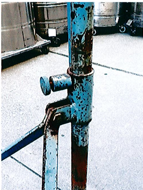
Latch that keeps the cart from folding.
