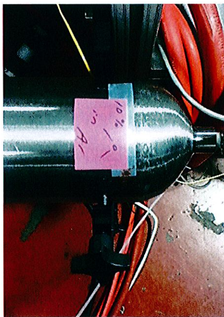
Custom engineered metal mount for cylinders. Cylinders are held at both ends securely.
