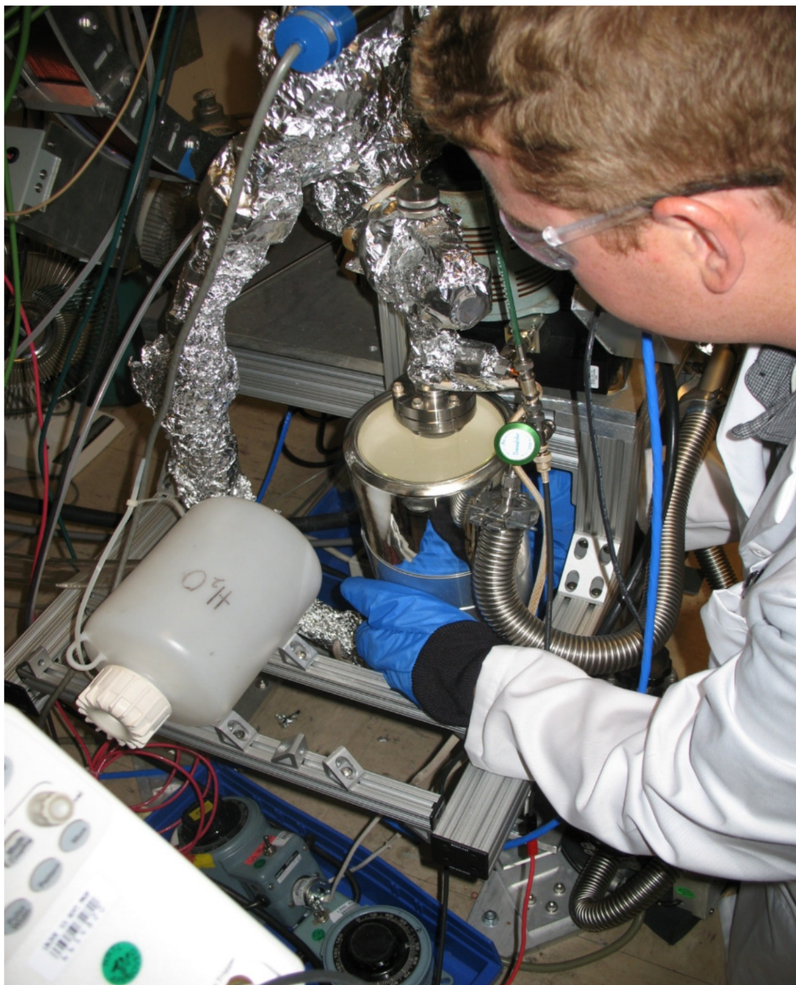
Picture 7. Introduction of filled and fully attached sample into either liquid nitrogen or dry ice.
