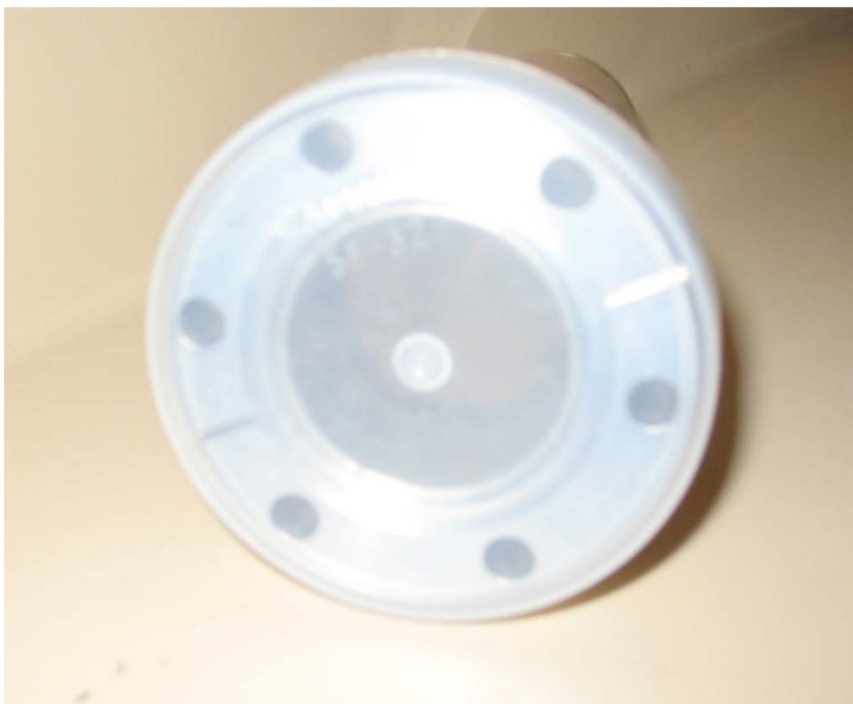
Picture 3. End On view of sample holder. Six hole attachment flange
